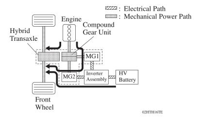
• When more engine power is required, in order to increase the engine speed, the rotation speeds of the related gears change as follows. The directions in which the torque acts on each gear are the same as those described in "During Low Load and Constant-speed Cruising".
