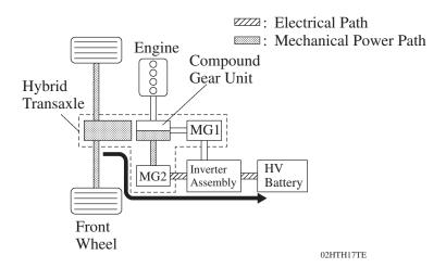
• During deceleration, the ring gear is rotated by the rear wheels. Under this condition, due to the engine being inactive, the rotational speed of the carrier is 0 rpm. In addition, since MG1 does not generate any torque, no torque acts on the sun gear. However, the sun gear (MG1) rotates freely in the (–) direction balancing the rotating ring gear (Output).
