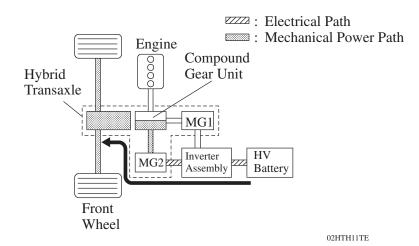
• When the vehicle starts off under normal conditions, it runs using the motive force of MG2. While running under this condition, the rotational speed of the carrier is 0 rpm due to the engine being inactive. In addition, since MG1 does not generate any torque, no torque acts on the sun gear. However, the sun gear rotates freely in the (–) direction balancing the rotating ring gear (Output).
