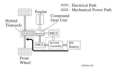
• The conditions of the planetary gear are opposite to those described in "Starting and Running with MG2". Due to the engine being inactive, the rotational speed of the carrier is 0 rpm but the sun gear (MG1) rotates freely in the (+) direction balancing the rotating ring gear (Output).
